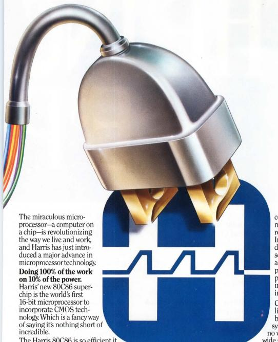
The Harris 80C86 is so efficient it offers the same high computational performance as other 16-bit processors with up to 90 percent reduction in power consumption. As a result, it can run for weeks on miniature batteries. It generates substantially less heat, too, thus promoting longer equipment life.
