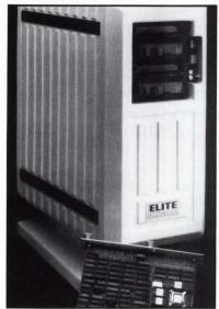
The latest member in a family of 32-bit multiprocessor computers, the Expert 32 supports up to six processor cards. Based on the NS32032 CPU, each processor card includes a floating-point processor, a memory management unit, and 32 kbytes of cache memory.
