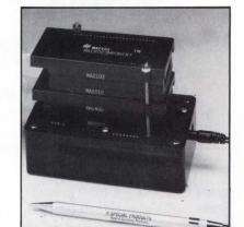
tery backup and is portable and readily configured, since it has no backplane and consists of stacked modules. With Forth, the system can be easily programmed for test, diagnostic, control, and datalogging operations.
