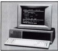
modified version of the IBM 5531 industrial computer, the Macsym 120 workstation adds an 8087 math coprocessor, Concurrent CP/M-86, and multitasking MacBasic to optimize operation. Additionally, Macsym I/O cards support more analog channels (as many as 30 on a single card) than any other IBM-compatible plugin cards. For distributed applications, Macsym front ends provide analog and digital interfacing.
