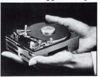
Intended for use with personal and portable computers, a 3½-in. Winchester disk drive is designed to tolerate a wide variety of adverse environmental conditions. The micro-Winchester, designated the HP 97501A, is able to withstand shocks of up to 50 G without requiring elaborate mounting techniques. It also withstands 95% relative humidity and rapid changes in temperature.
