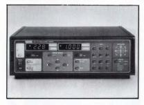
eaturing an IEEE-488 interface, the Model 228 programmable bipolar source can sink or source 100 W in either a constant-current or a constant-voltage mode. The instrument's nonvolatile memory is capable of storing operating parameters for up to 100 different test setups. To accommodate a broad range of test applications, memory sequencing can be controlled over the 488 bus or via the unit's front panel.
