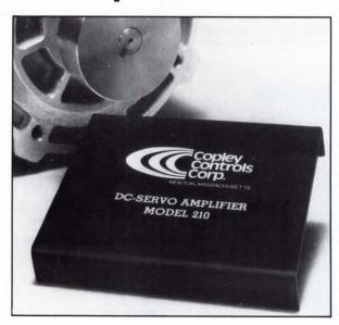
and the circuitry needed to operate in a rate loop or as an inner loop in a position control system. It delivers 4 A continuously or 10 A for 1 second at 75 V, operating at a switching frequency of 22 kHz and therefore eliminating essentially all audible noise.
