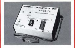
**EPROM PROGRAMMER Model EP-2A-79** with software for the Atari, TRS-80 (1&3), Pet, Apple, AIM-65, SYM-1, VIC-20, C-64 Ohio Scientific, H-8, H-89, SS-50, and S-100, Programs 2708, 2716, TMS2716, 2732, 2732A, 2532, 2764, 2564, 27128, and MCM68764 EPROMS; 2816 EEPROM; 8751, 38E70 MPU, Price \$169 with personality modules \$17 to \$35, Software \$19 to \$40, Optimal Technology, Earlysville, VA, 22936, 804-973-5482.
