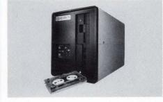
Heurikon presents Minibox, a multiuser UNIX<sup>™</sup> workstation based on the MC68000/68010 and Uniplus + <sup>™</sup> UNIX System III or V. Minibox supplies its users with six Multibus substantial slots, floppy disk drive, interactive streamer tape drive and up to 420 Mbytes of storage in one compact and attractive cabinet. Contact Heurikon Corp., 3201 Latham Dr., Madison, WI 1-800-356-9602.
