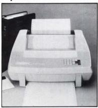
The SX dot-matrix printer offers multiple modes of operation to provide draft, near-letter-quality, and letter-quality printing at speeds of up to 300 char/s.
